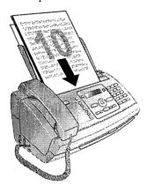
2 Then configure the desired resolution. You can choose between RESOL.: STANDARD (for documents without special features), RESOL.: FINE (for texts with small print or drawings) and RESOL.: PHOTO (for photos). Press . The configured resolution appears on the display. Press again to change the resolution
