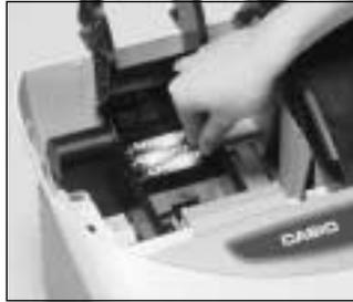
3. Note the (+) and (-) markings in the battery compartment. Load a set of three new SUM-3 (UM-3) batteries so that their positive (+) and negative (-) ends are facing as indicated by the markings.
