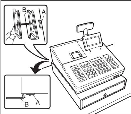
1. Thoroughly clean the location where the fixing angle bracket (B) is to be placed.
