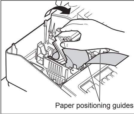
4. Feed the end of the paper along with the paper positioning guides as per the diagram.
