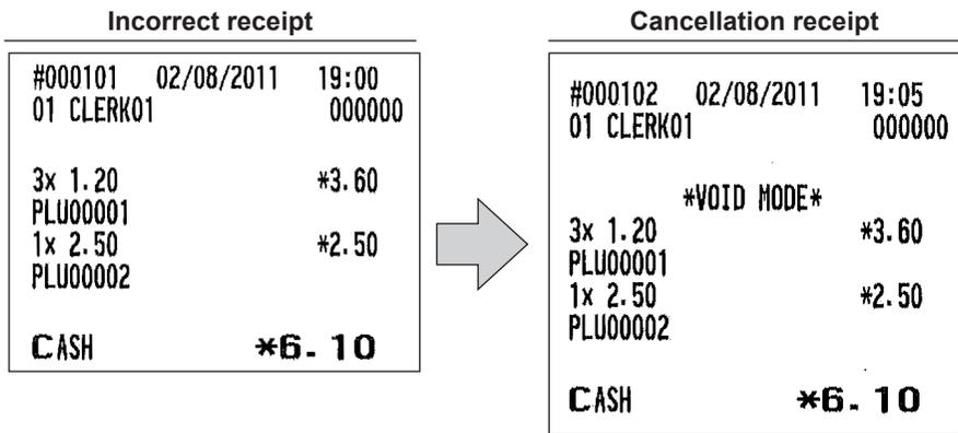
**NOTE** Your register leaves the VOID mode whenever a transaction is canceled (i.e. finalized in the VOID mode). To void additional transactions, repeat steps 1 and 2 above.
