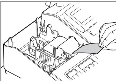
6. Cut off the excess paper and replace the printer cover.
