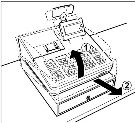
1. Lift up the front of the register and pull the register towards you.
